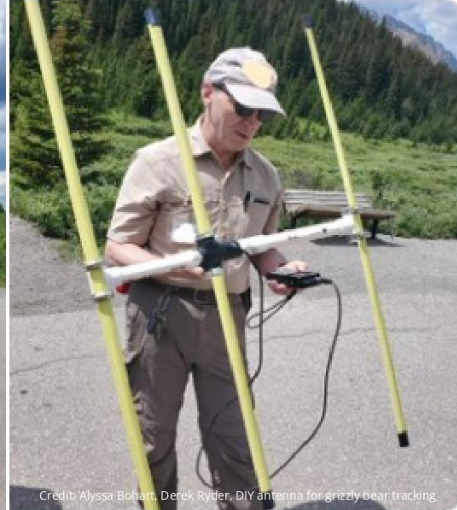
Credit: Alyssa Bohart, Derek Rylier, DIY antenna for grizzly bear tracking
